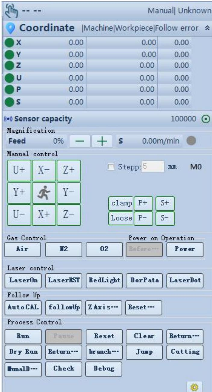
a) Coordinates (coordinates of machine tool movement axis can be observed)
